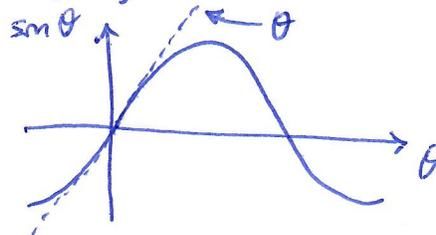
Then a linear approximation to the pendulum dynamics is:
